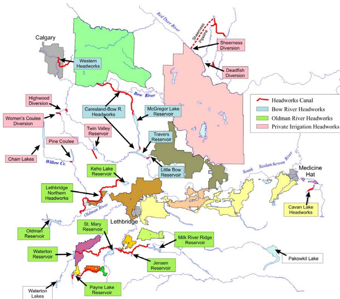
Figure 5: AENV water diversion and storage facilities supporting irrigation within the SSRB
